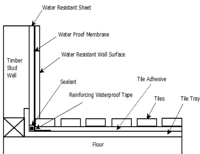
After installation onto the substrate, apply downward pressure and check the tile tray is level.
