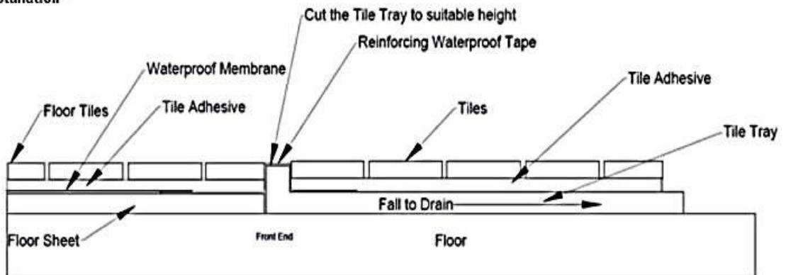
The waterproof membrane should extend at least 1500mm from centre of the tile tray outlet. The fall of the floor outside the tile tray must be towards the tile tray outlet to comply with local standards.
