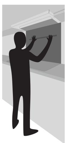
When pressing your SS panel against your Polymer splashback use a spirit level or straight edge to ensure a nice even flat contact.
